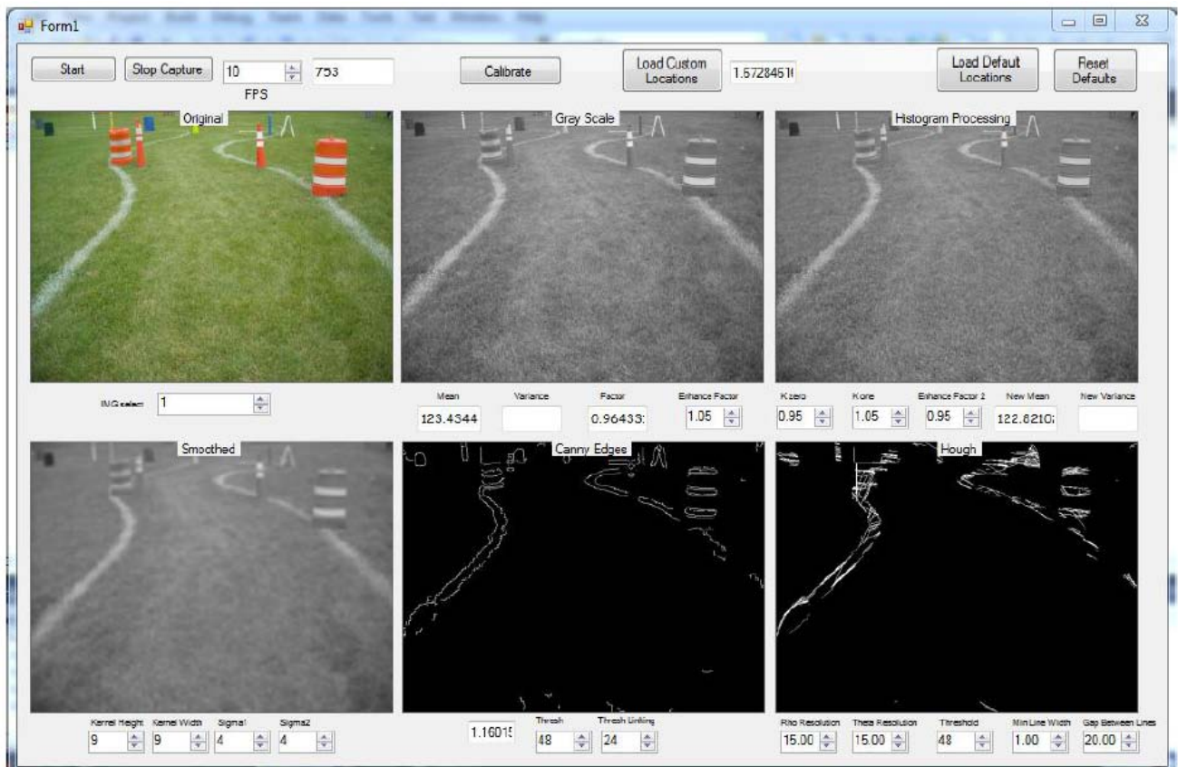
Figure 3: Visual Depiction of Image Processing Flowchart (Top to bottom, left to right)
